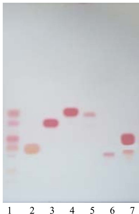
Fig. 1. The chromatograms in the conditions of amino acids identification. 1 – the 1 st sample solution in ethanol (10% v / v); standard solutions of amino acids in ethanol (10% v / v): 2 – glycine, 3 – valine, 4 – leucine, 5 – tyrosine, 6 – aspartic acid, 7 – glycine and glutamic acid.
